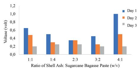
Figure 5. Bioelectrolyte voltage measurement results
