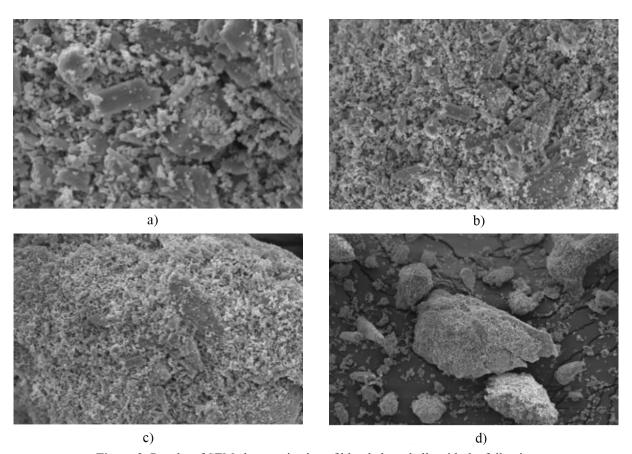
**Figure 2.** Results of SEM characterization of blood clam shells with the following magnification: (a) 10 000×, (b) 5000×, (c) 3500×, (d) 1000×
